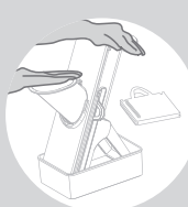
Adjust thickness pad, front side for 2 mm, back side for 4 mm.
